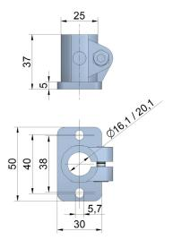
■ Flanschklemmstück 20-AL, flange clamp material: aluminium, temperature resistant up to 120 °C
