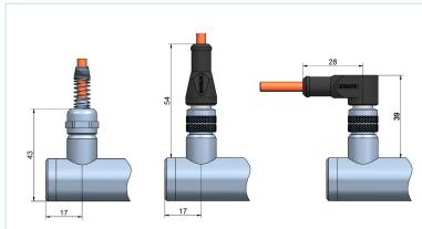
For sensors with connector output the cable has to be ordered separately. You can choose from a cable with a straight connector or with an angular connector. The connector is protected from accidental removal by a threaded fitting (M12). When bolted, the connector pair has the protection class IP67.
