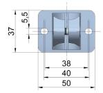
Fußklemmstück 16-VA / 20-VA, base clamp material: stainless steel, temperature resistant up to 200 °C
