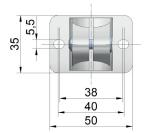
Fußklemmstück 16-AL, base clamp material: aluminium, temperature resistant up to 120 °C
