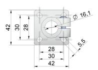
Fußklemmstück 20-AL, base clamp material: aluminium, temperature resistant up to 120 °C
