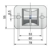
Flanschklemmstück 16-AL, flange clamp material: aluminium, temperature resistant up to 120 °C
