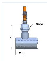
Sensors with cable output have a cable fitting and a spring for bend protection of the cable. For installation, the bending radius should not be less than 3 times the cable diameter. The standard cable length is 2 m.
