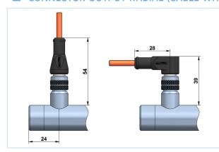
For sensors with connector output the cable has to be ordered separately. You can choose from a cable with a straight connector or with an angular connector.
